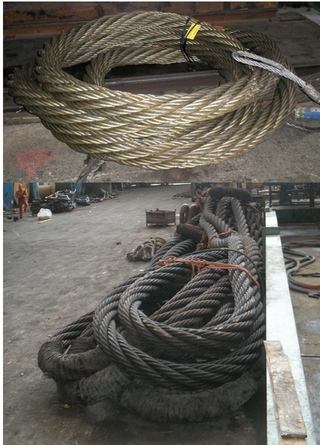
Cross section cable laid slings and grommets
