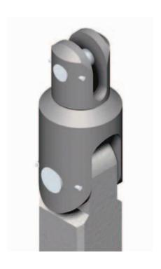
The POOL® superbox swivel is the shortest possible approved connection between anchor and chain. Application of the POOL® superbox swivel means a shorter distance between anchorshank and chain stopper. The winches can be placed more to the front of the vessel, which reduces the required deck area. The POOL® superbox swivel can be connected directly to the anchorshank. No crownshackle is required.
