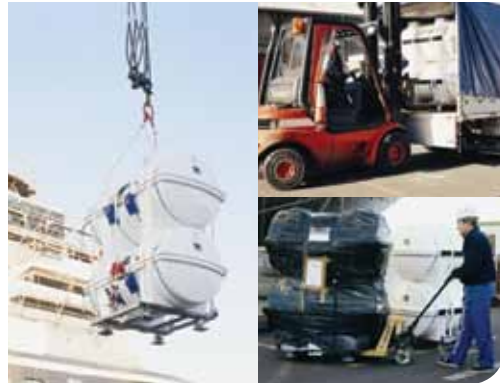
DELIVERED PRE-FITTED ON THEIR DECK CRADLE, THE LIFERAFTS BECOME EASILY PORTABLE DURING INSTALLATION OR REMOVAL FOR SERVICING BY EITHER A PALLET JACK OR FORKLIFT
