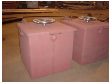
Central closed tank hatch
